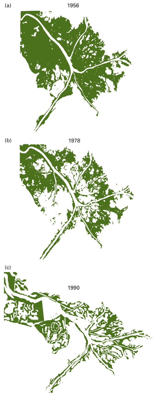
Figure 6.31 Comparison of the outlines of the Mississippi Birdsfoot Delta from the 1930s to 1990 gives a clear indication of the transformation from marsh to open water. Artificial controls upriver have decreased the amount of sediment carried by the river; artificial levées along much of the lower course have kept flood-borne sediment from replenishing the wetlands, and in the active delta itself, rock barriers installed across breaks similarly confine the river. The Gulf of Mexico is intruding as the marshland sinks or is washed away.
