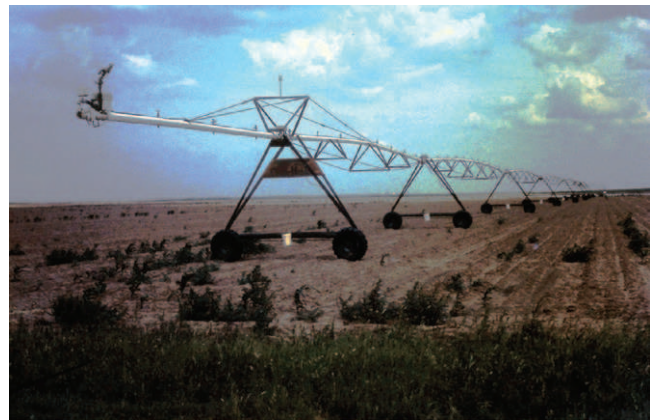
Figure 5.17 In the High Plains of the USA, fields are irrigated by centre-pivot irrigation schemes which use groundwater. Groundwater levels have fallen rapidly in many areas because of the adoption of this type of irrigation technology. (See Plate 36)
