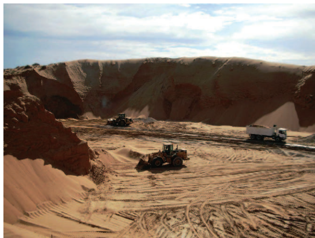
Figure 6.2 The mining of sand from large linear sand dunes to provide material for the construction industry in Dubai, United Arab Emirates. (See Plate 38)
